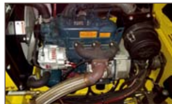
Turbo engine 44 hp to amplify extra power
