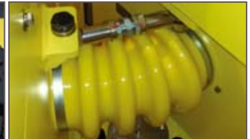
Double articulation with lubrication points 'Pac - pivot' (patented)
