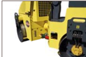
Double articulation with lubrication points 'Pac - pivot' (patented)
