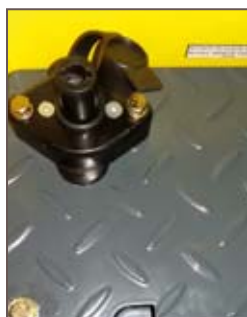
Anti-theft central locking mechanism
