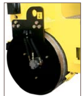
Poclair hydraulic system. Casappa vibration system.
